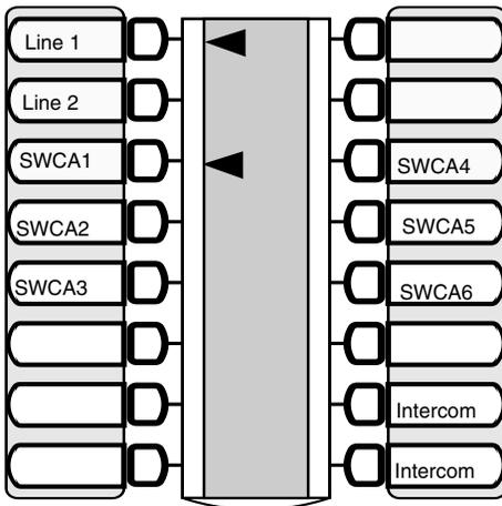
In this example, the call comes in on line 1 and automatically assigns to SWCA1 (the first available SWCA button).
