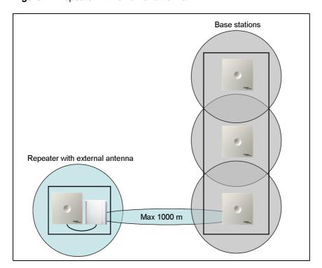
The digital repeater relays the radio signals between the handsets and the base station, making it a wireless component from the DMC.
