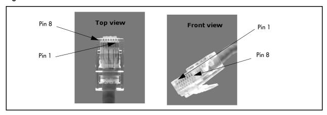
Table 10 DMC - RJ45 connection diagram
